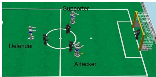
Fig. 10. Example of roles in offensive attacker tactic. In this case attacker shoots the ball to opponent goal.
