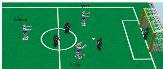
Fig. 11. Example of roles in offensive attacker tactic. In this case attacker shoots the ball to supporter. If supporter catches the ball, he becomes new attacker and shoots to the opponent goal.
