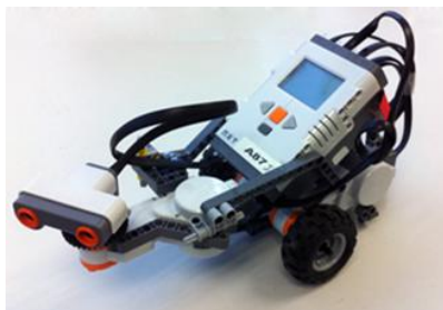
Figure 2: LEGO Mindstorms NXT in differential drive configuration.
