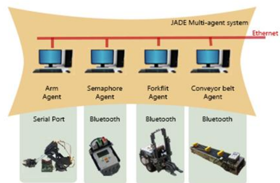
Figure 10: Architecture developed for the industrial environment application.
