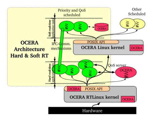
Figure 4-2. OCERA Architecture, hard and soft real-time support
