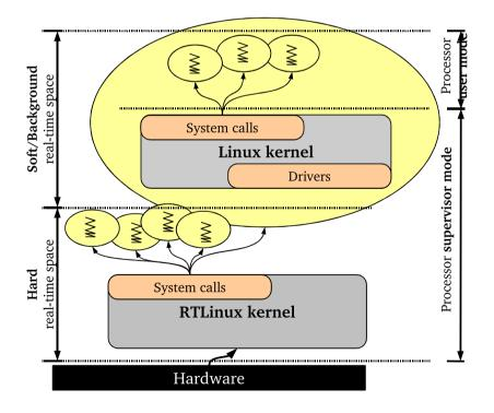
Figure 2-2. Different view of the execution environments
