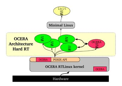
Figure 4-1. OCERA Architecture, hard real-time support
