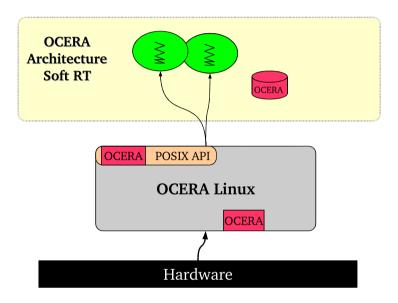
Figure 4-3. OCERA Architecture, soft real-time support
